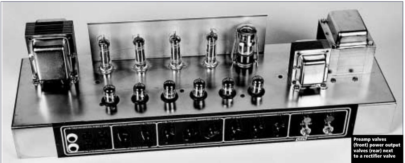
Preamp valves (front) power output valves (rear) next to a rectifier valve
